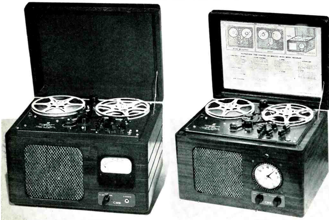
Fig. 1 (left). Brush BK-401 magnetic paper-tape recorder adapted for broadcast recording applications. The standard illuminated type VI is mounted at a slight angle to give good visibility with the VI selector-switch and earphone monitor jack mounted below it. The VI amplifier chassis is located behind the VI meter inside the cabinet. In the unit shown, the VI is used only for recording as only a low-level playback output is provided. However, where the output circuit is arranged to feed a transmission line directly, a fourth switch position may be provided to enable VI and earphone monitoring of "line" output. Fig. 4 (right). Brush BK-401 recorder adapted for automatic operation in home or office installations. The recorder and a radio receiver associated with it may be operated normally with the auto-manual switch set to "manual" as shown. With this switch set to "auto", they may be automatically operated to record any two 15-minute periods as preset on the built-in clock/timer. The playback/radio switch enables either the recorder playback output or the normal radio signal to be fed to the receiver audio amplifier and loudspeaker.
