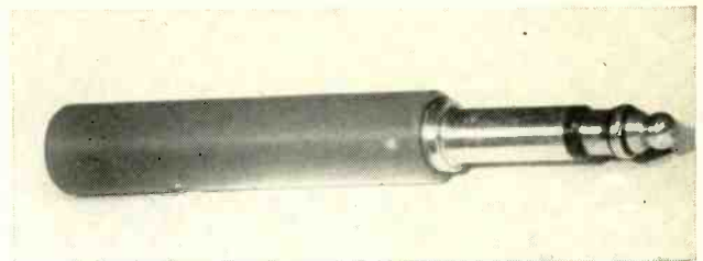
Fig. 3. A tip, ring, and sleeve type of single plug often used in telephone switchboard work. This type of plug is not satisfactory for use in audio systems as explained in text.
