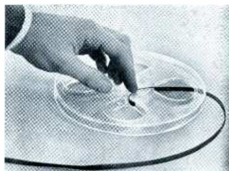
B. Drop tape into slot, leaving about 1 inch projecting beyond the hub with tape slack on both sides of recording head. Then press the "start" button. Tape will grip and hold firmly . . . no need to turn reel by hand to anchor free end.
