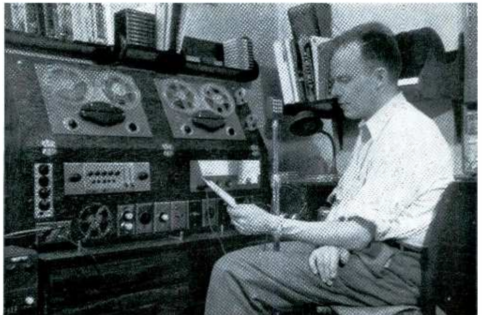
Dr. Adolph G. Dittmar, General Co-ordinator of UFO Information Service, sitting at the control panel of his home studio. To keep up with the heavy recording traffic of his post "Ditt" has: two Fen-Tone Brenell 3-speed tape decks, a Fisher master audio control, a Fen-Tone PRO2 recording amplifier, a Fisher 80 AZ 30-watt audio amplifier, and a monitoring system complete with speaker and amplifier. A red light on the outside of his studio door lends a professional atmosphere to the New York branch of UFO Information Service.
