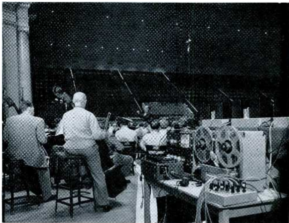
WGMS-Soundorama rehearsal from backstage, showing part of the recording setup using Berlant BR-1 recorders with 10½-inch reels of Audiotape, 10 Fisher 50AZ amplifiers and 10 Jensen Imperial speaker systems.
