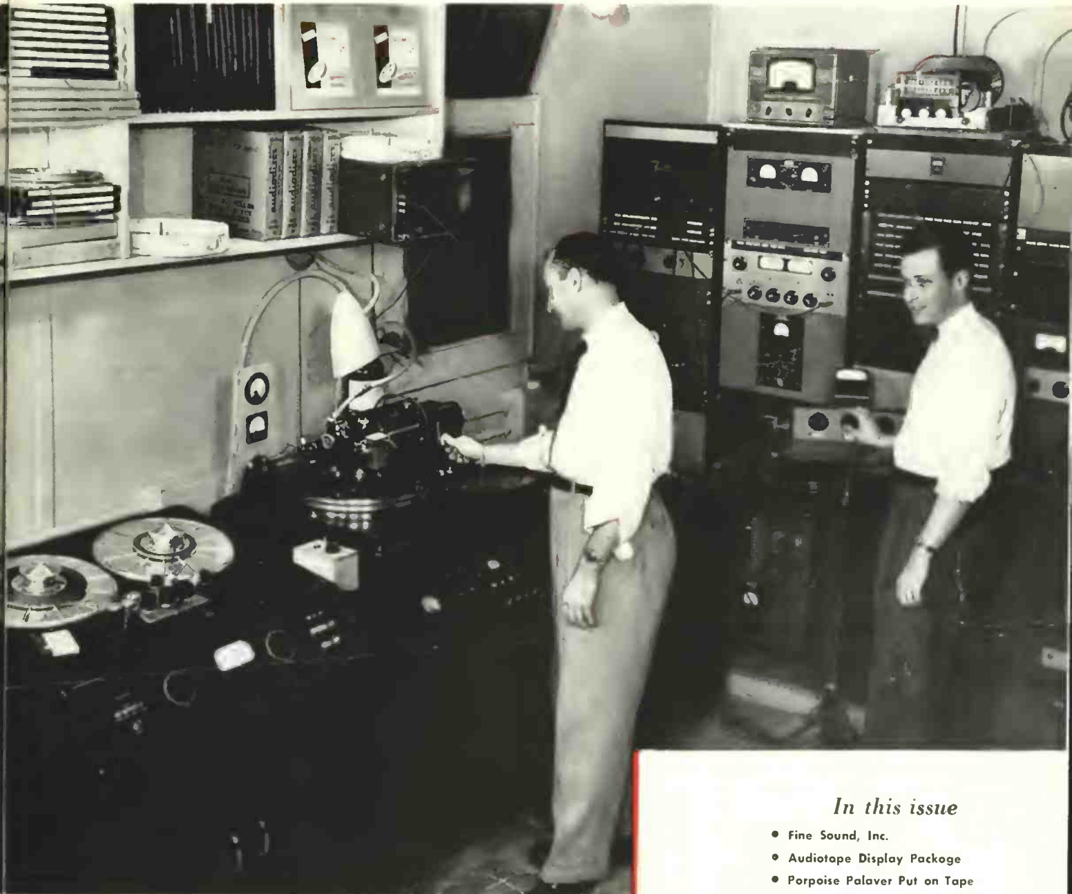
Fine sound in the making, by Fine Sound, Inc. George Piros (left) tends the Margin Control while cutting a long playing master, as Bob Fine (right) adjusts the recording level. Equipment shown includes a Fairchild tape recorder and Fairchild Model 523 Disc Recorder with Miller cutterhead specially made to Fine Sound specifications. Story on Page 2.
