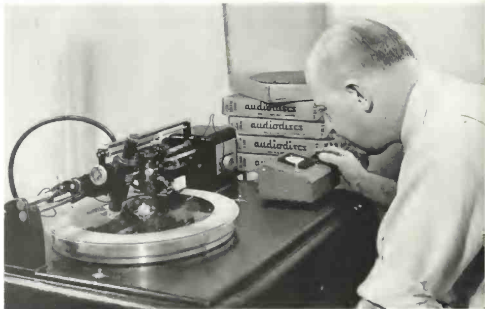
James S. Stewart, Chief Engineer of Recorded Publications Laboratories, cutting a phonograph record master on one of the Fairchild variable pitch lathes with Thermo-Stylus.
