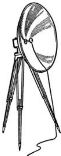
Fig. 4.5 A parabolic reflector with centrally mounted microphone.
