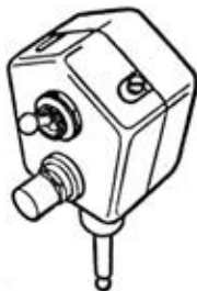
Fig. 1.4 A radio jack with a two-position station selector switch. Some radio jacks are constructed to receive three stations.
