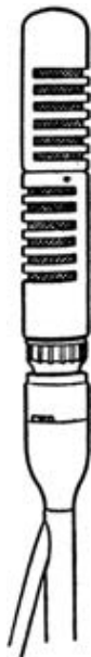
Fig. 5.2 A dual-purpose microphone consisting of two bi-directional units mounted above each other and capable of being used together or as a stereophonic pair.
