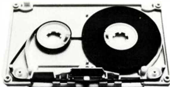
Cassette with the lid off. This BASF Special Mechanics cassette embodies improvements designed to ensure free running of the tape.
