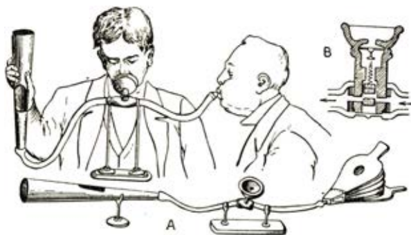
Fig. 7-1. (A) Edison's aerophone, or pneumatic amplifier, provided a sound transmission channel into which additional energy was injected in the form of compressed air. Inset (B) shows how the sound-actuated valve throttled a steady flow of air, to create an instantaneous variation in flow that imitated the original sound vibrations.
