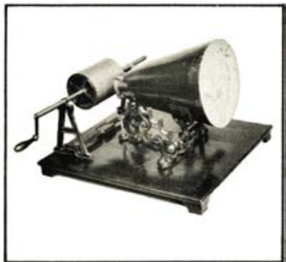
Fig. 3-1. The phonautograph of Léon Scott de Martinville—a commercial sound recorder of the eighteen sixties. (Courtesy Smithsonian Institution)
