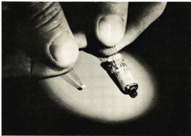
Fig. 7-5. The junction transistor is tiny compared to the "sub-miniature" tube, the smallest type made. These are approximately full size. (Courtesy General Electric Co.)
