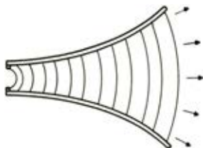
Fig. 12-6. Increase of effective radiating area of a small diaphragm at the throat of a horn to the area of the mouth.
