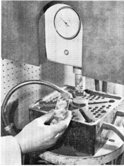
Drilling germanium slices to form circular base wafers
