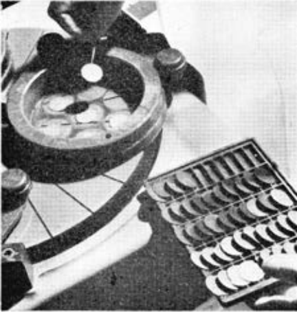
Removing slices of germanium crystal after lapping
