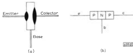
Fig. 2—(a) Simplified cross-section of transistor (b) Simplified 'block diagram' of transistor
