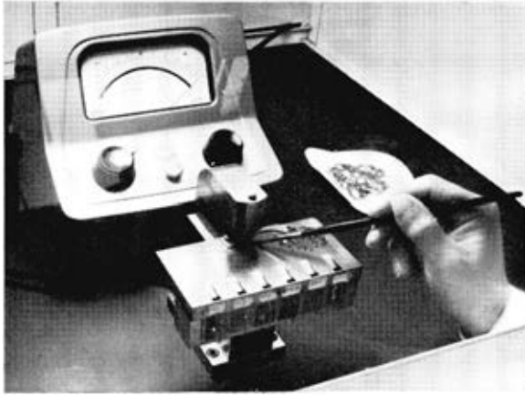
Measuring the thickness of the base wafer prior to alloying. An electronic method of measurement is used, accurate to \pm 0.5\mu\text{m}
