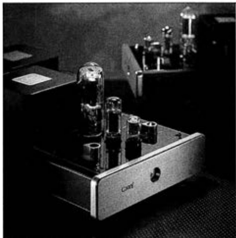
Last year's Cary 805 sans 300B driver, but still capable of showing what genuine SE triodes can do.
