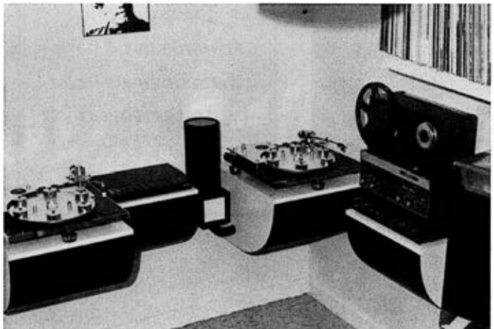
Jimmy's system circa 1974: Transcriptor Hydraulic Reference turntables, SME 3009i and Fluid arms, Lecson AC1/AP1 amps, Gale GS401A speakers and no wire!
