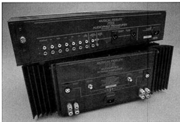
The F22 preamp offers six line inputs, but one of these can be configured for use as either a moving magnet or moving coil phono input.
