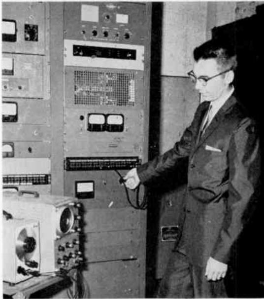
Engineer completes final inspection of multiplex transmitting equipment at WKFM, Chicago. This station is one of the first to schedule FM stereo broadcasts on a daily basis.
