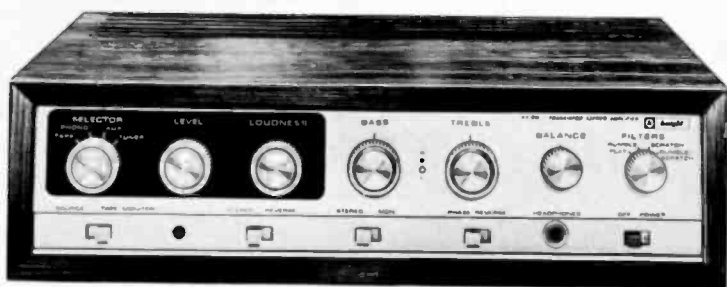
Fig. 3-1. This dual channel (stereo) amplifier with built-in preamplifier has inputs and controls for all program sources (Knight-Kit KG-870).
