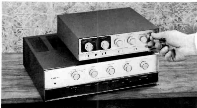
Fig. 3-4. Size comparison between stereo amplifier using vacuum tubes and comparable transistorized unit.
