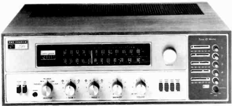
Fig. 2-4. Multiplex FM-AM stereo receiver (Fisher 250T). Dual amplifier and FM-AM stereo in one compact case.
