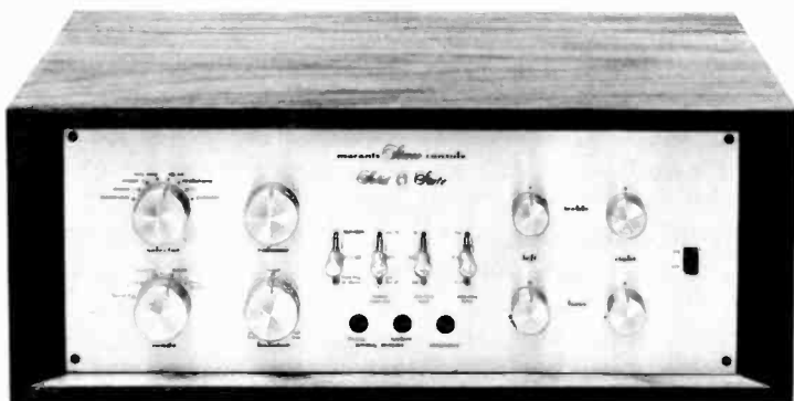
Fig. 3-3. Stereo preamplifier (Marantz 7T).
