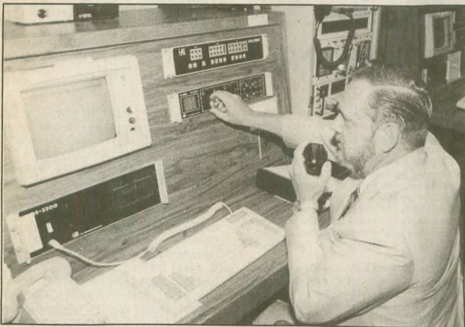
Army MARS Chief, Bob Sutton, speaks with an overseas MARS operator while setting up a phone patch. MARSgrams are typed into the computer on the console in front of him and can be viewed on the monitor before being transmitted.
