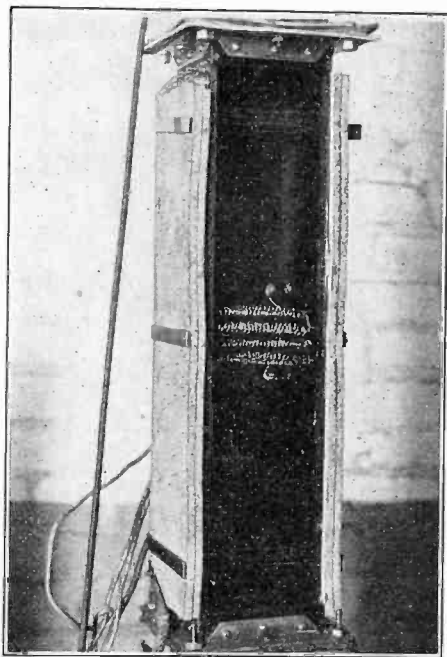
FIG. 1—A SMALL VOLUME METER WITH ONE SIDE REMOVED FOR INSPECTION
