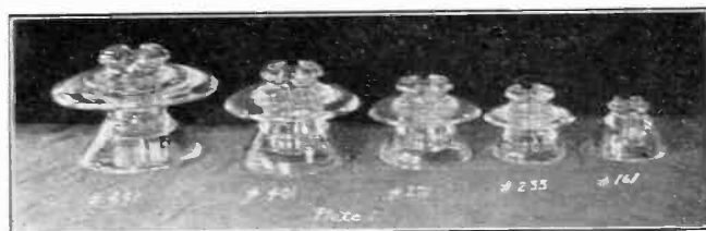
FIG. 1—PYREX INSULATORS USED IN TESTS
