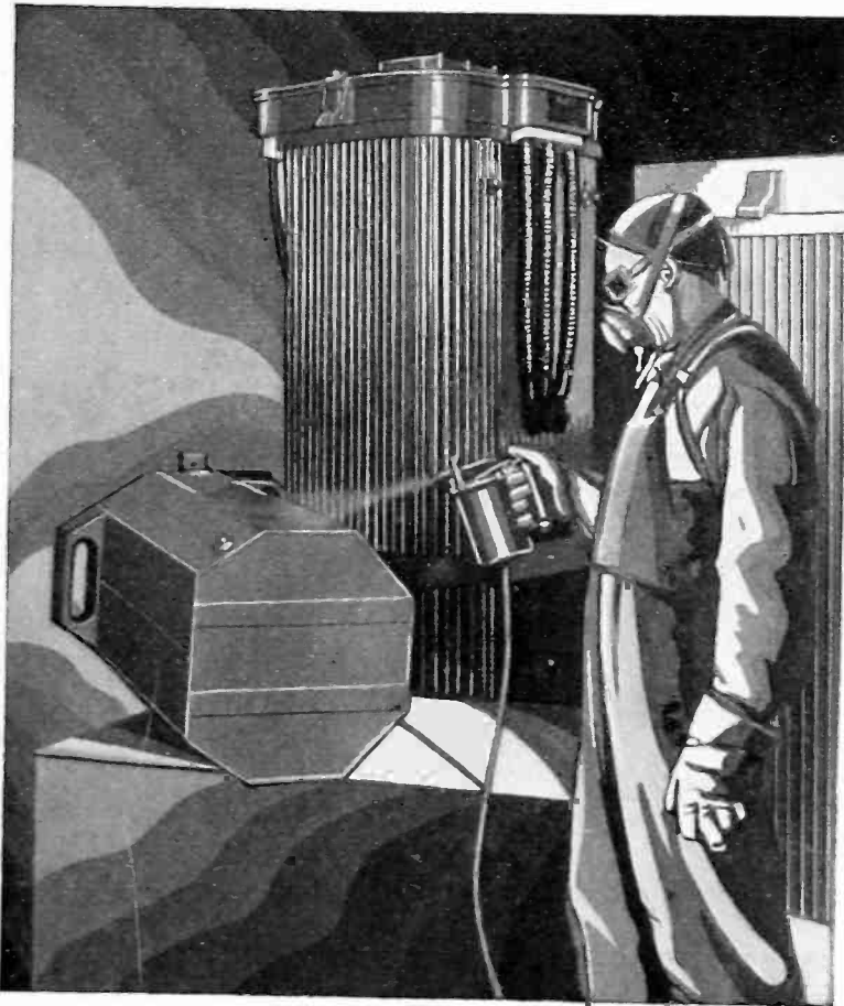
Spray gun method of painting transformer cases with battle-ship gray paint. Note iron skids on bottom of the case.
