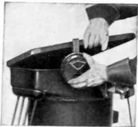
Showing method of installing pole-type thermotel
