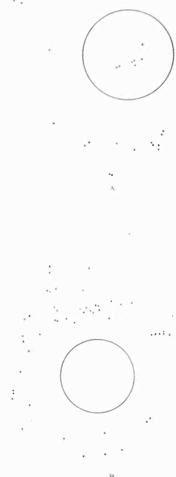
FIG. 14—TARGET MADE BY LIGHTNING STROKES FROM CHARGED CLOUD
