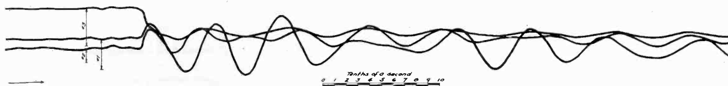
FIG. 10—OSCILLOGRAPHIC WATTMETER RECORD OF CLOSING ONE LINE Stability Tests at Pit River Power House No. 1, June 18, 1925, 12:12 a. m. El. No. 1—No. 1 Gen. Power No. 2—Hat Creek Power No. 3—No. 1 Line Power
