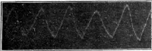
FIG. 8—FILM 8-A VIB. NO. 2-3W., NO. 1 MACHINE FULL LOAD. 60 CYCLES TIMING WAVE
