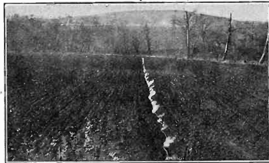
FIG. 10—EFFECT OF GROUND ON 66-KV. LINE WIRE
