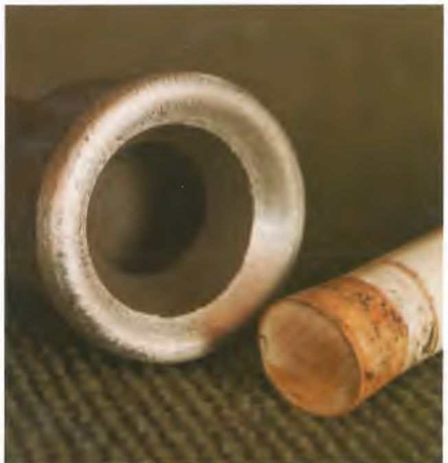
New yoke and insulator with flared end.
