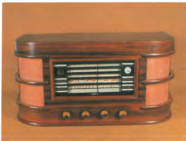
HMV seven valve bandspread wooden cabinet mantel receiver imported from New Zealand 1947.
