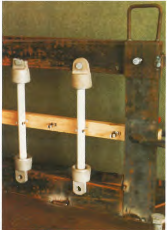
Jig for holding insulator during encapsulation.
