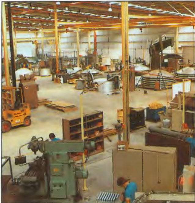
A view inside the plant showing the spinning machine in the foreground with spun reflectors nearby.
