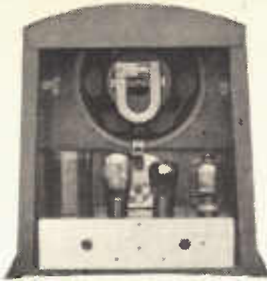
Looking from the rear of the set, showing the speaker in the cabinet.
