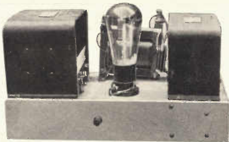
Looking at the power pack from the front, showing the rectifier inserted in its socket.
