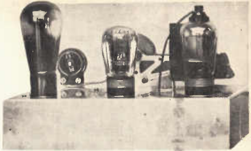
A back view of the receiver with the valves inserted in their sockets.
