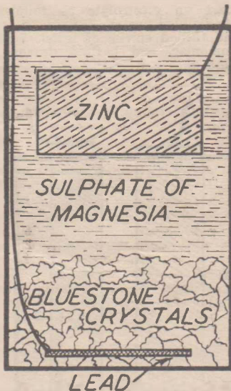
Diagram of a Gravity Cell.
