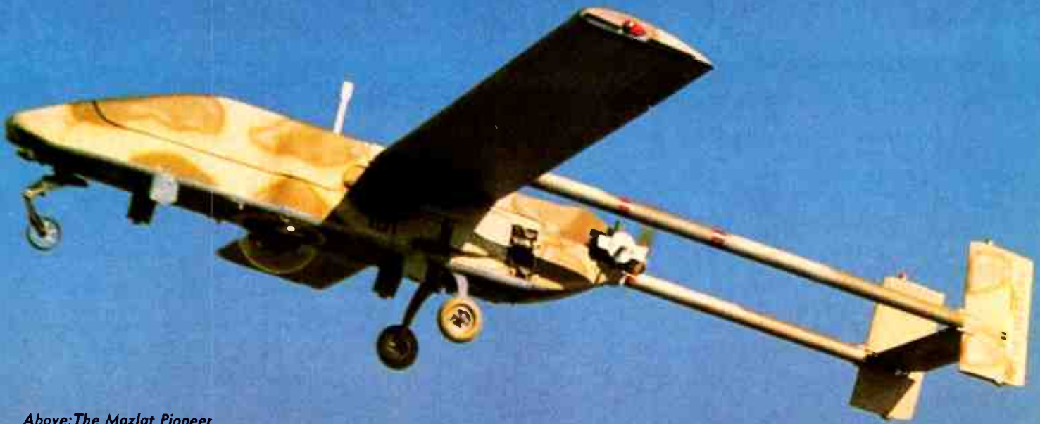
Above: The Mazlat Pioneer remotely piloted vehicle is used for reconnaissance and target practice.
