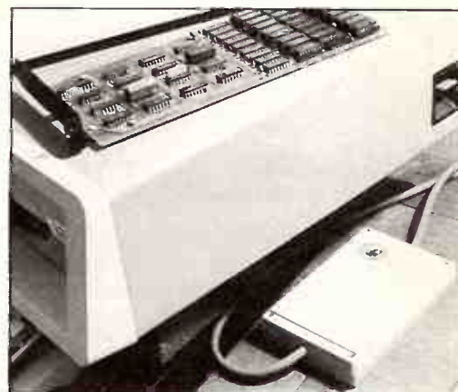
Figure 7 Your humble author would never switch on the IBM-PC without this power line filter in the 240 V line.
