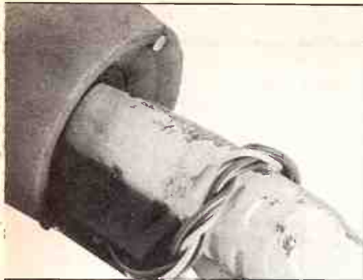
The skateboard wheel, showing the magnet located in the rubber at top and the Hall Effect Switch mounted on the chip carrier at bottom.
