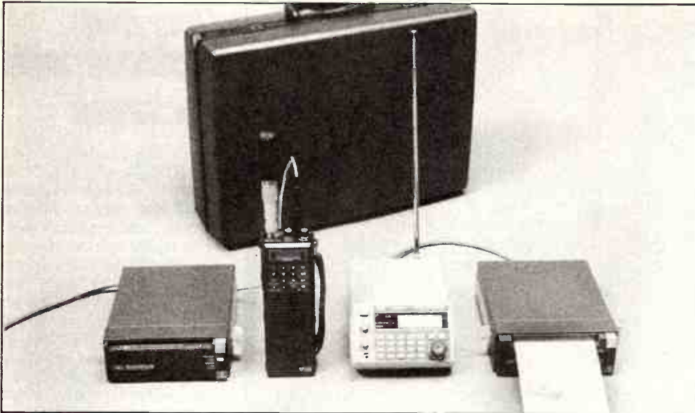
JRC's dashboard mountable fax equipment able to transmit images 104 mm wide puts mobile communications in the forefront.
