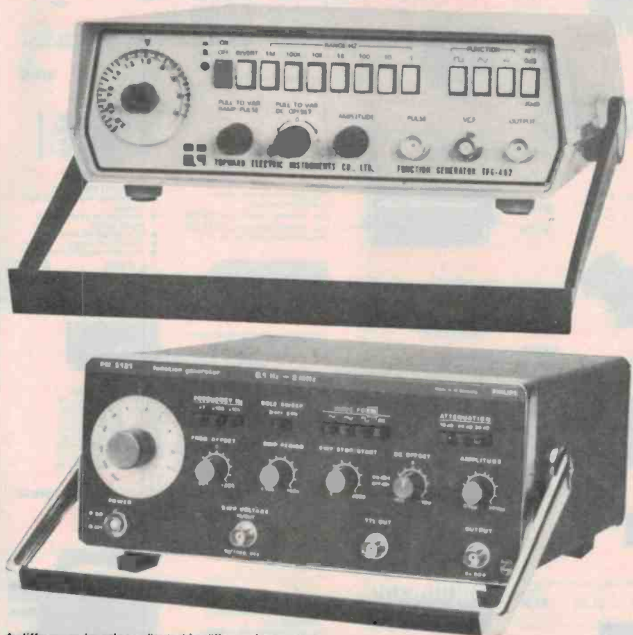
A difference in price reflected in different features. The PM5131 has fewer waveforms but faster rise time, higher output voltage and sweep period.
