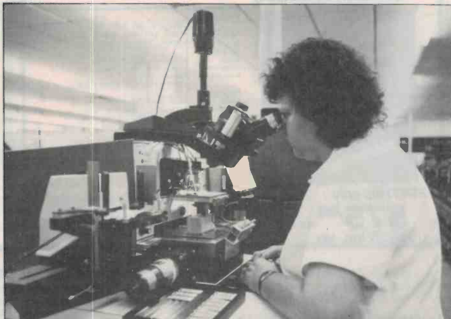
Through the looking glass. The silicon chip is connected to the substrate via fine wire lines. These are held, positioned and glued by the micro-manipulators she is controlling.
