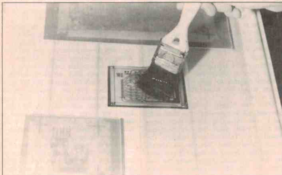
Turn the board over and use a fine (25 mm) brush to get fine detail.
