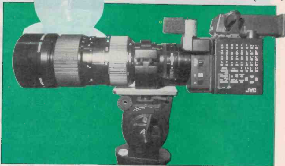
Tiny, but oh so versatile. JVC's new VHS-C camera takes standard 35 mm camera lenses and features an add-on character generator for titling. ▶
