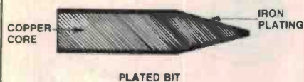
Figure 5. Plated bits last longer because they do not oxidise as rapidly as unplated bits. They are usually iron-plated.
