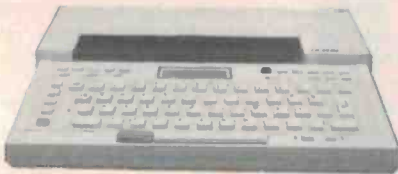
EP-44. A revolutionary typewriter from Brother with a display that shows the last 15 characters as they are typed. It also has a Centronics socket on the side so it functions as a printer. The keyboard would not please a professional typist but it is excellent for a 'peek and poke' merchant. Print quality is disappointing given the other advanced features.
