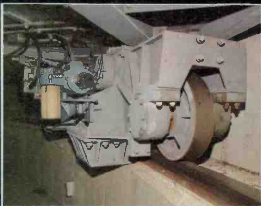
Below. Building drive. The building rides on four bogies, two of which are fitted with dc electric motor-drives, like this one.
