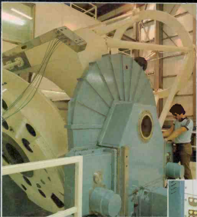
Below. Building drive. The building rides on four bogies, two of which are fitted with dc electric motor-drives, like this one.
