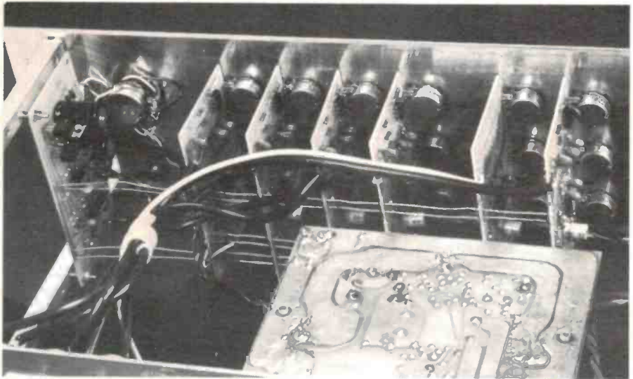
Below. View of rear panel (from top of case), showing wiring routing to sockets on the rear panel.
