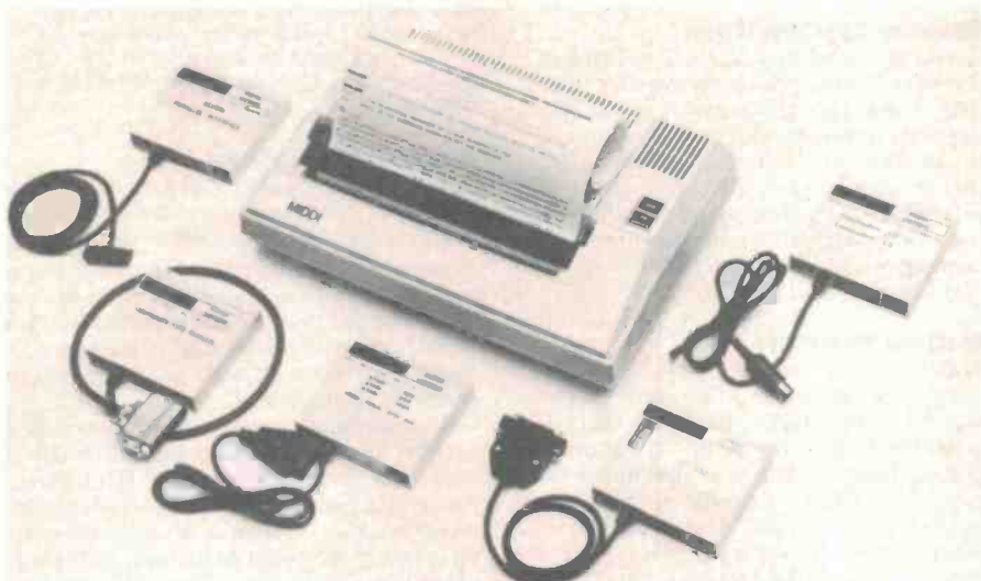
Interfacing. One solution to interfacing. The boxes contain an Intel 8049 processor programmed to carry out the conversion from the computer's protocols to something the printer can handle. The printer here is an Alphacom M1d1. (From Oscwell International.)
