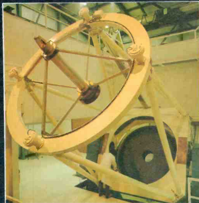
Down the barrel. View from the top-end of the telescope. The four electric motor-driven top-end clamps are clearly visible. The primary and tertiary mirrors are not in place here.
