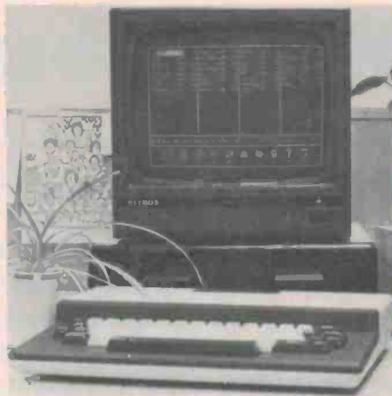
64K Z80 & 6502 CPU IBM look-a-like case detachable keyboard 188 function keys, 10 user define keys $480
