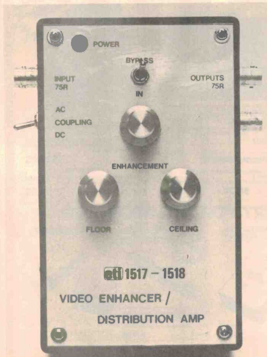
Controls. The enhancement control works between the limits set by the floor and ceiling controls.
