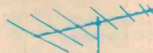
Figure 5. A typical log-periodic beam antenna (horizontally polarised here). All the elements are split in the centre and 'cross-connected' to the next in line.
