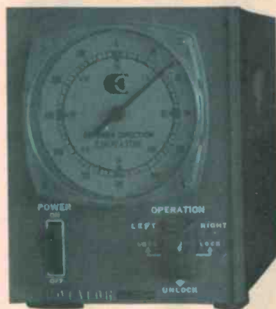
Beam rotator. A typical beam rotator comprises a motor housed in a weatherproof enclosure (to which the beam is attached) — on the right — and a remote control and Indicator unit — on the left — sited at your operating position. This is the Emotor 103SAX, available from G.F.S. Electronic Imports, Melbourne.
