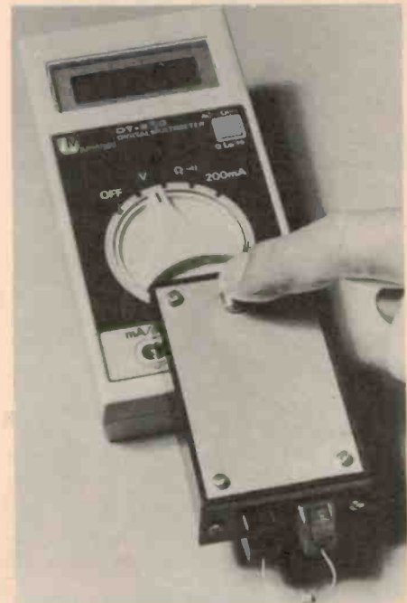
Push-to-read. The tester is housed in a 'zippy' box with banana plugs protruding from the rear spaced to suit the multimeter input sockets spacing.
