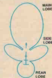
Figure 6. The 'radiation pattern' of a typical beam antenna, showing how the sensitivity varies to signals from different directions. To pick up a signal from a particular direction, the antenna is rotated so that the main lobe points in the desired direction (where the signal will be strongest).
