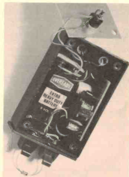
Inside story. Internal view of the zener tester. Note the cut-down banana plug handles at the top of the box.
