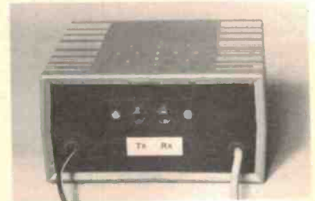
In and out. Rear view of the Interface showing the ac input line at left, the RCA sockets for connections to the transceiver and the cable to the line at right.
