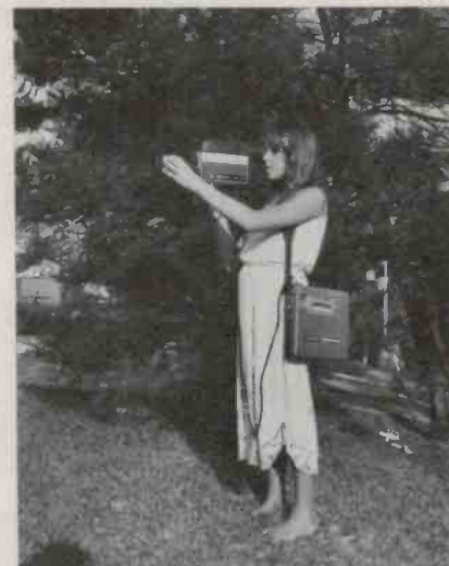
The 3 kg VCR is small and light and can be used with any standard video camera.
