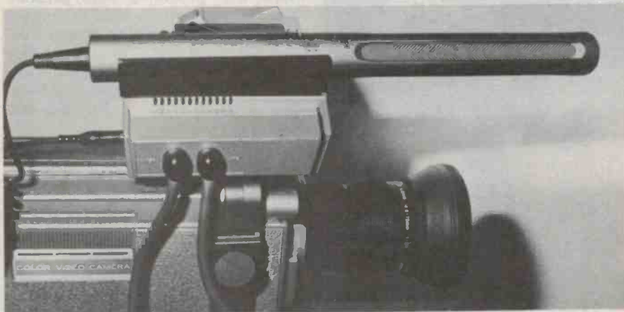
No, it's not a weapon in the video war, but it's certain to become involved in the battle! The picture shows JVC's zoom mic that clips onto your video camera so you can zoom in on the sound when you zoom in on the picture.
