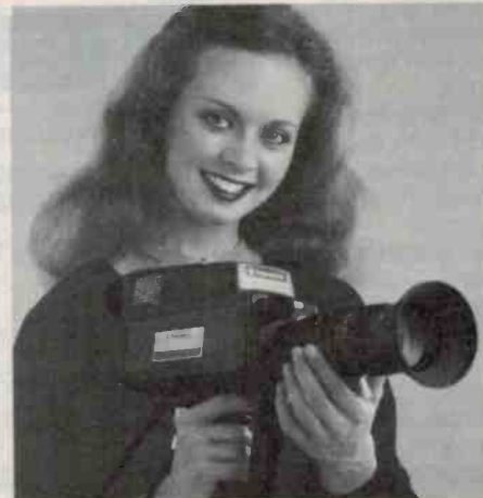
National's WV3300E features their high resolution 'Cosvicon' tube, a standard 6:1 zoom lens and electronic viewfinder.
