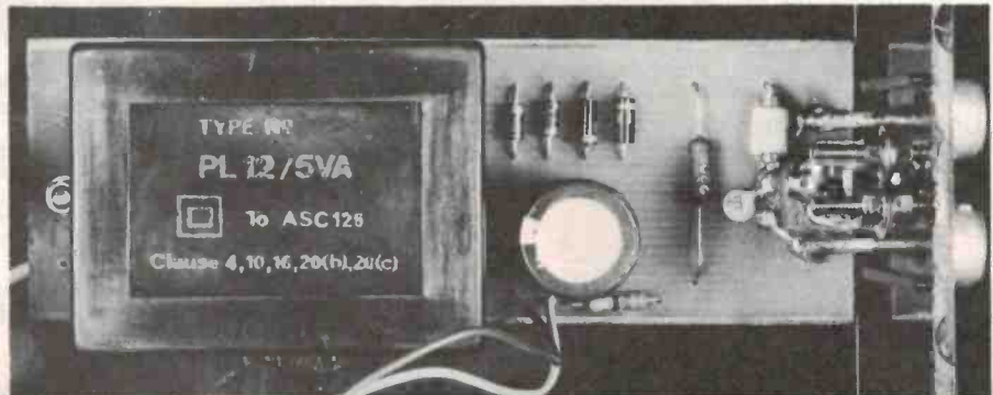
Internal view of the power supply. Note the pc board is double-sided.
