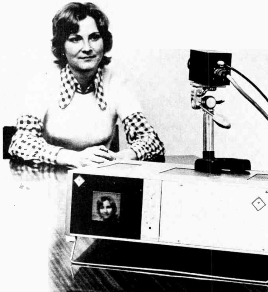
Fig. 13. Although not primarily intended to rival conventional C.C.T.V. (at this stage of development) a useable picture can be formed with a 64 x 64 array. The reconstruction is made on a C.R. Tube.
