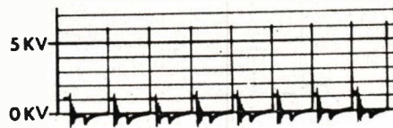
Firing lines even but high: Excess plug gaps, rotor gap, break in coil ht lead, mixture too lean ignition retarded.
