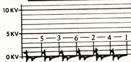
Normal pattern: Note that the firing line for cyl. 1 appears at the extreme end of the trace. The remaining cylinders then appear in engine firing sequence.
