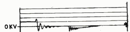
Unusual point opening signal (note hash extreme right of picture) burnt or arcing points.
