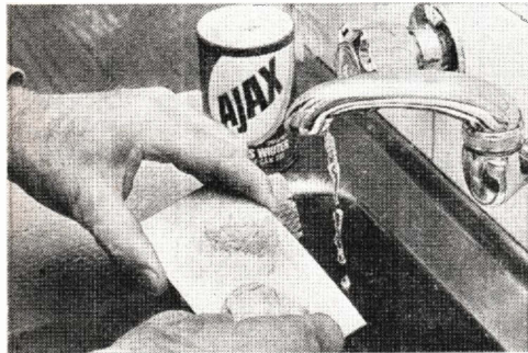
The laminate should be thoroughly cleaned with paper towel and abrasive cleanser powder until the surface is uniformly bright, and wets uniformly.
