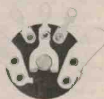
Fig. 3. A miniature, transistor-radio style pot. It is generally mounted firmly to a printed circuit board or other suitable support with bolts through the large lugs.
