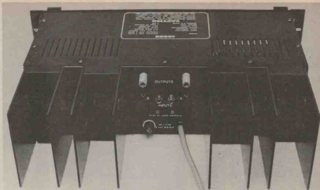
The output transistors are mounted under four covers located at the bases of each pair of cooling fins.
