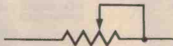
Fig. 13. Pots in some applications require only a variation in resistance. Which terminals are connected together depends on the circuit effect.
