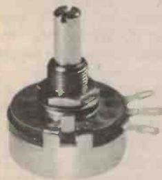
Fig. 1. The common, basic style of potentiometer. It has a threaded bushing and nut for panel mounting through a single hole and standard solder lug terminals.
