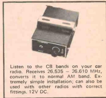
Fig. 6. A CB converter. This model comes from Dick Smith for $33.
