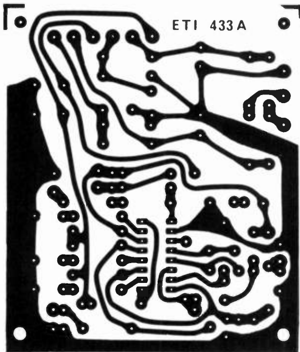
Fig. 5. Printed-circuit layout for the two-way board. Full size 77 x 90 mm.
