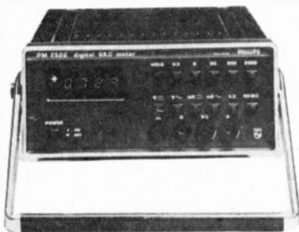
PM 2522: LED display. Optional rechargeable batteries high reliability. Full circuit protection
