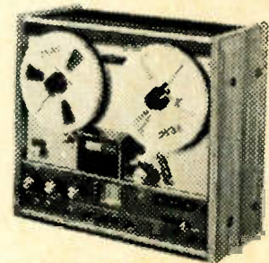
Stereo Tape Deck Model A-1230 ● 3 heads-4-head function ● Reel size 7" ● Tape speed 3¼ ips and 7½ ips ● Triple motor mechanism ● Wow and flutter .08% at 7½ ips ● F/R 30 to 22,000 Hz at 7½ ips ● S/N Ratio 55dB
