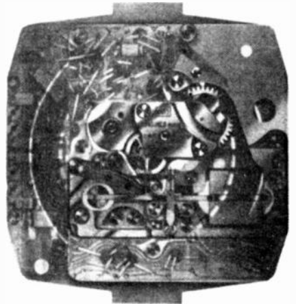
Fig. 5. SWISS-CEH — The Swiss Centre of Electronic Horology developed this movement for a number of member companies including Bulova and Omega. It uses an 8.192kHz oscillator and five stage IC divider to produce 256Hz which is fed direct to a motor. Gearing provides the remaining step down.
