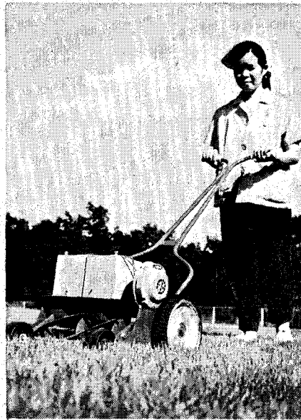
Fig. 9. This electrically powered lawnmower uses a printed circuit motor drive.
