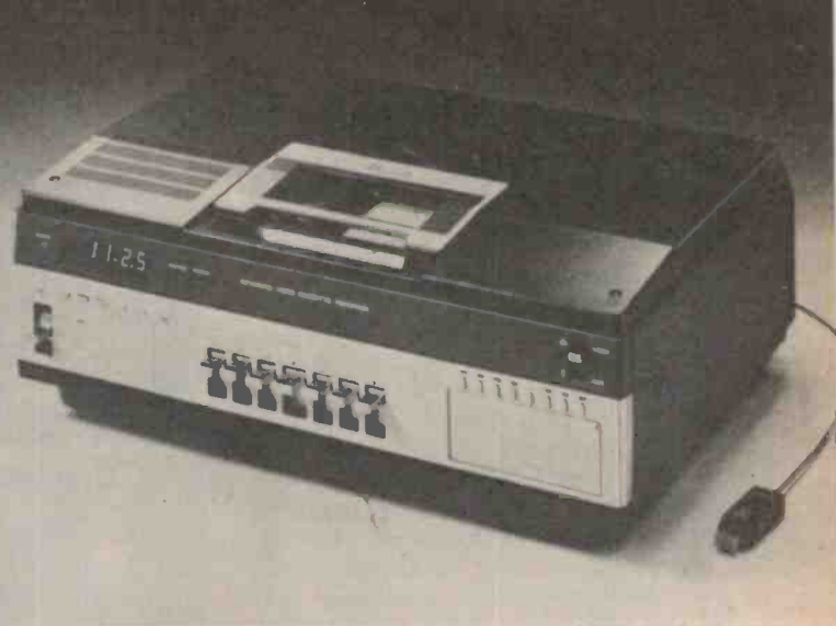
Sanyo claim their VTC 9300 is one of the best-selling VCRs in Australia today. Using the Beta format, it can play for up to 3¼ hours.
