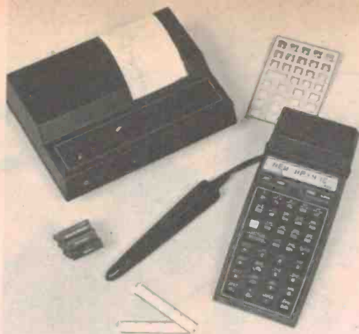
ABOVE: The HP-41C with printer and assorted peripherals. RIGHT: At top are examples of the special character capabilities, while beneath is portion of a sine plot.
