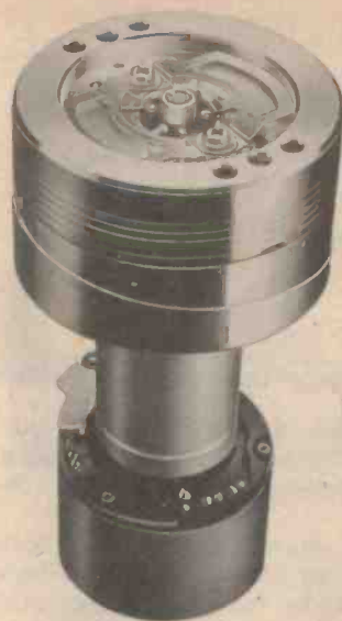
The mechanical precision and finesse necessary in video cassette recording machines is illustrated in the two pictures above. At left is a record/playback head, at right a tape guide and transport mechanism module.
