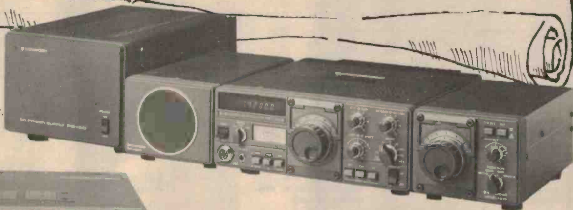
PS-30 20A Power Supply. SP-120 Speaker unit. TS-120S HF SSB Transceiver. VFO-120 Remote VFO unit.
