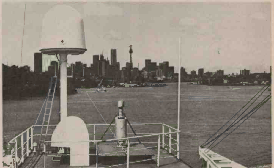
A close-up of the fibreglass radome which houses the above-decks antenna assembly.
