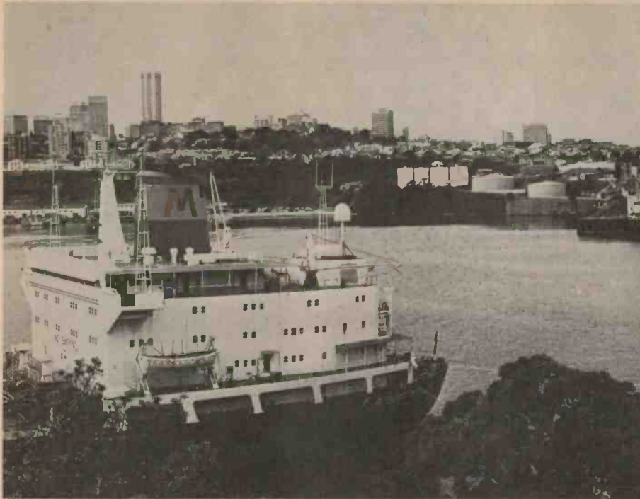
The Marisat antenna assembly can be seen above the stern of the Robert Miller, berthed at Sydney's Gore Bay.
