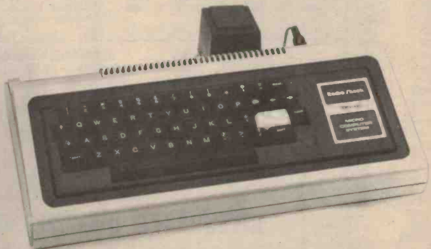
The actual computer, shown here, also incorporates a 53-key keyboard and VDU.
