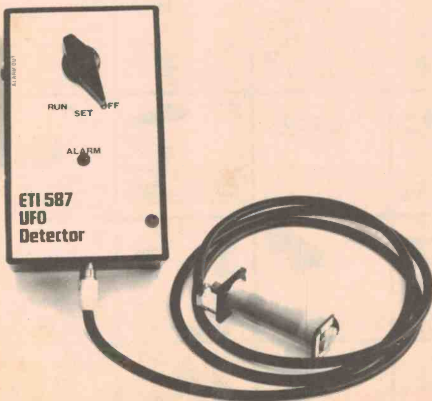
Fig. 1. The UFO Detector, attached to the solenoid.
