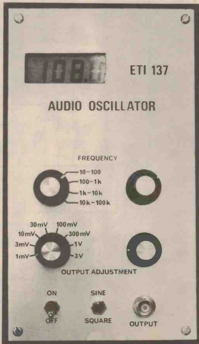
Front view of the audio oscillator. Note that this is an early prototype and the 3V range has been deleted.
