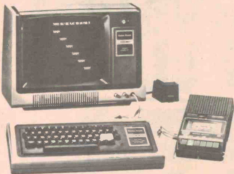
The four units which make up the complete TRS-80 microcomputer.
