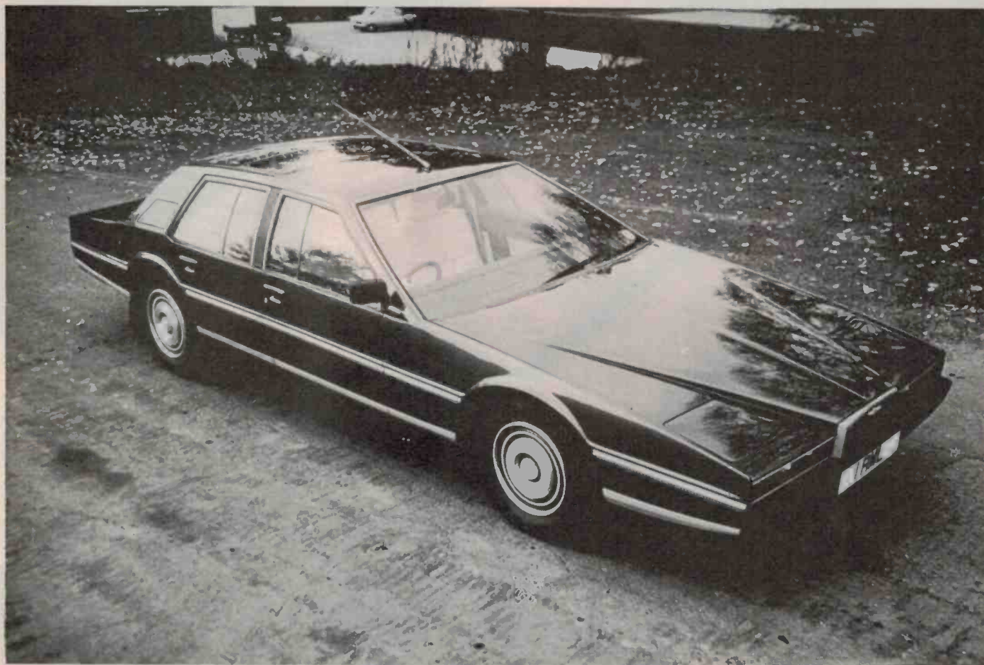
Fig. 10. The Aston Martin Lagonda features an integrated electronics system designed by Cranfield Institute of Technology and manufactured by a specially set up company, Aston Martin Electronics. Even the driver's seat is computer controlled through servomotors and can be pre-programmed with two sets of adjustments for husband and wife drivers. Extensive use is made of fibre optics in the control panel, which displays revs and speed in both analogue and digital forms. The speedo can be switched to read in either km/h or mph.
