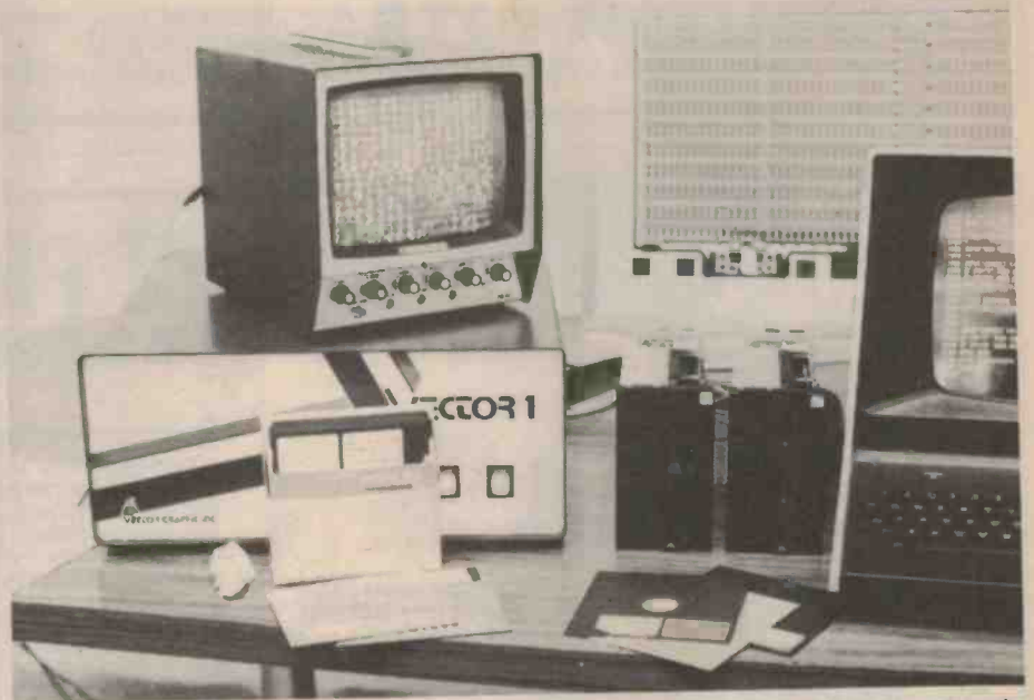
This is typical of the kind of system many small businesses are buying now, this one based on the Vector 1 microcomputer by Vector Graphics, with twin floppies and a terminal (or two).
