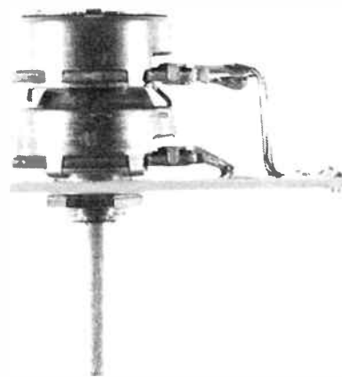
Showing how the dual-gang volume pot is wired to the front panel pc board.
