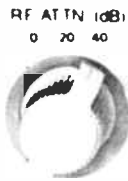
The 'RF attenuator' or 'RF gain' may be a continuous control, as at left, or a switch-type, as at right.
