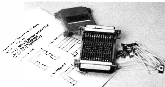
A low-cost RS232 patch box. This is the Arista 'mini patch box' where short links can be soldered between the required pin connections to test out a hookup. When it works, you just clip the lid on. It comes complete with brief instructions and suggested hookups. (Courtesy Geoff Wood Electronics).
