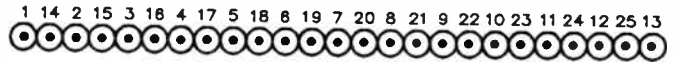
Figure 2. Numbering of the individual lines in a ribbon cable attached to an RS232 IDC connector.
