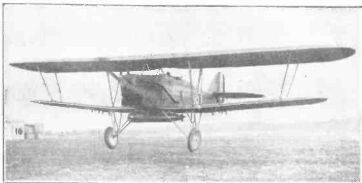
A Harker-Horsley standard day bomber and torpedo carrier of the R.A.F. A Rolls-Royce Condor engine is used.
